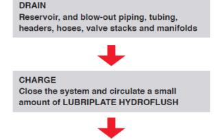
DRAIN SYSTEM Blow dry air, repeat step 7 if needed
